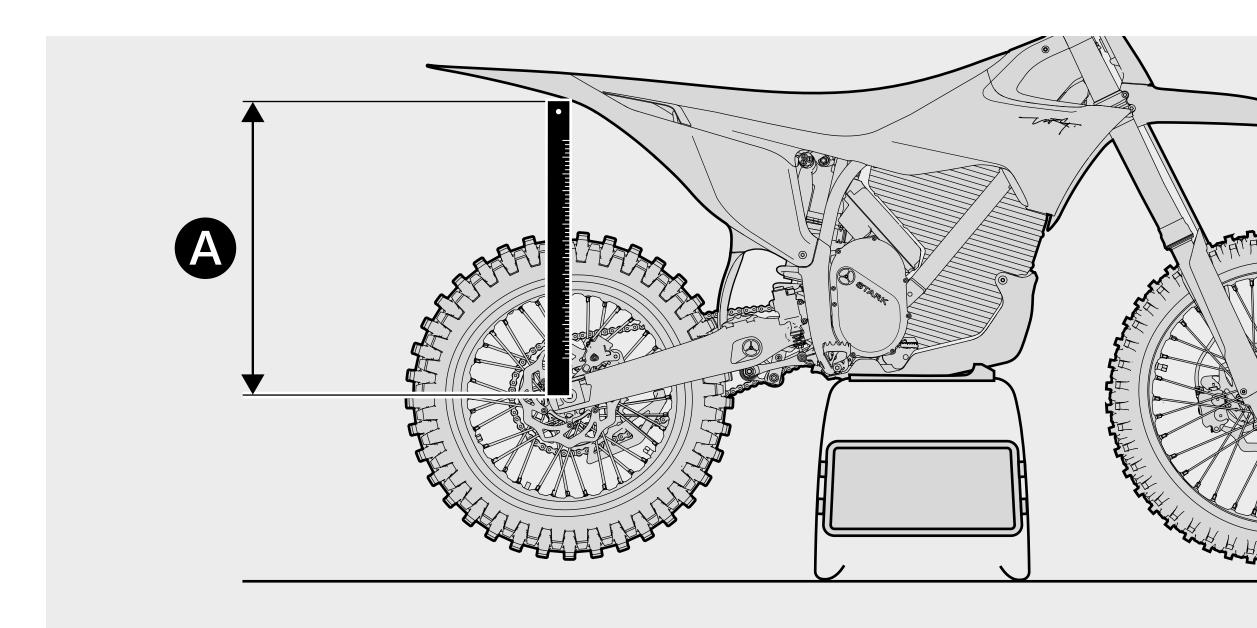
Measure the height A between the wheel axle and the SAG marking on the rear spoiler
