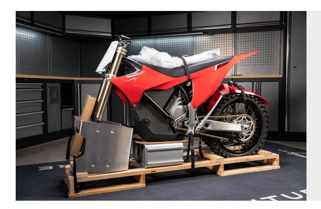
**3** Loosen the strap holding the toolbox and remove it from the **fork**.
