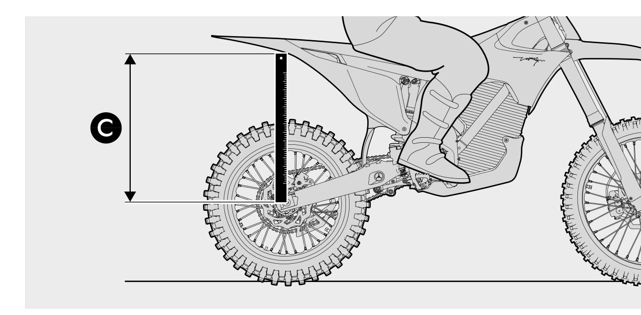
3 Place the bike with both wheels on the ground and, with a rider sitting on the bike, measure the height
