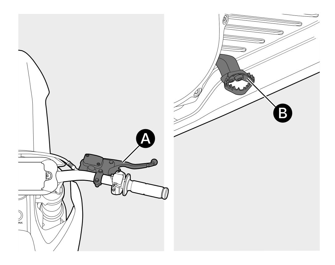
A Front brake B Rear brake pedal
