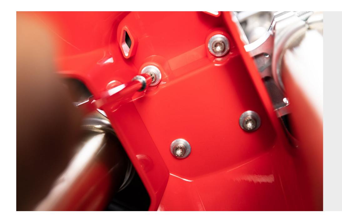
**39** Put the **front brake line** through the cable clamps on the back
