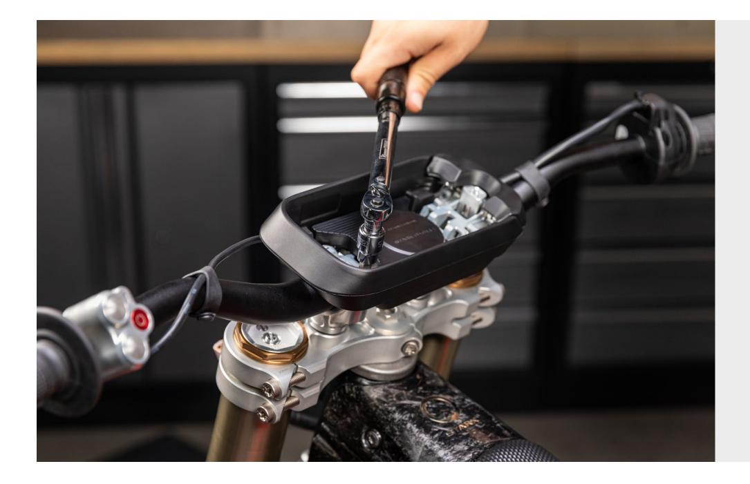
**11** Tighten the four bolts inside the **docking station** to 30 Nm.
