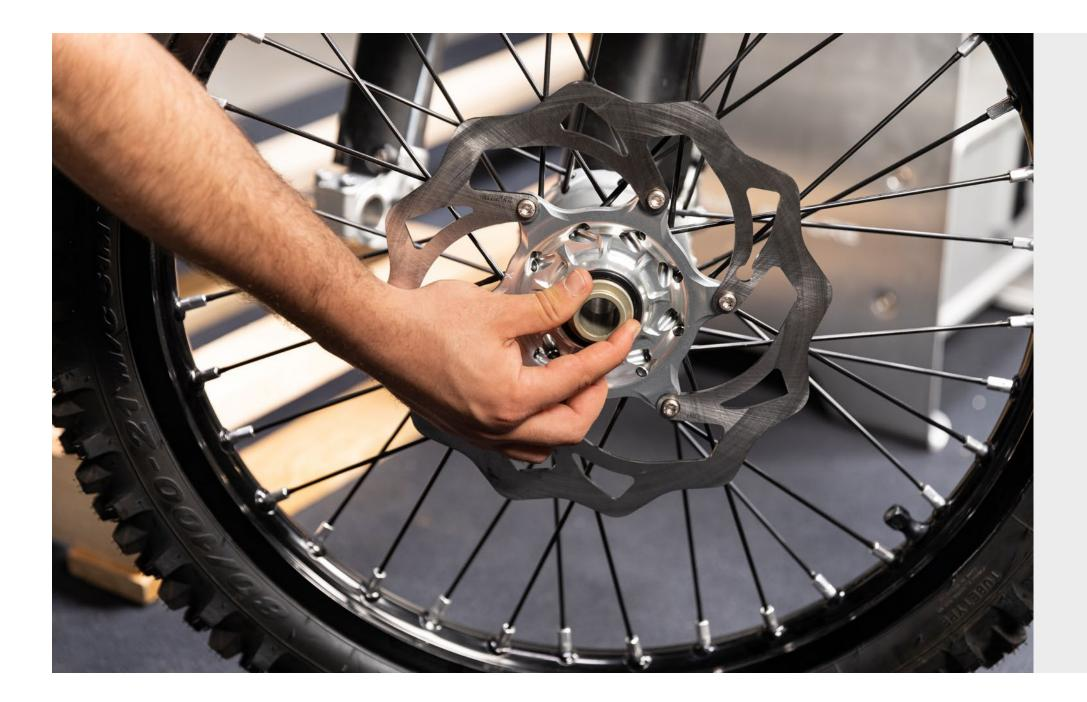
30 Place the front wheel with the spacers in between the fork protectors and align the shaft.
