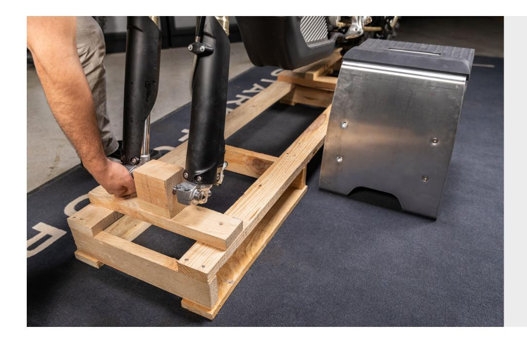
25 Lift the front of the bike and place it with the skid plate resting on the charger stand.
