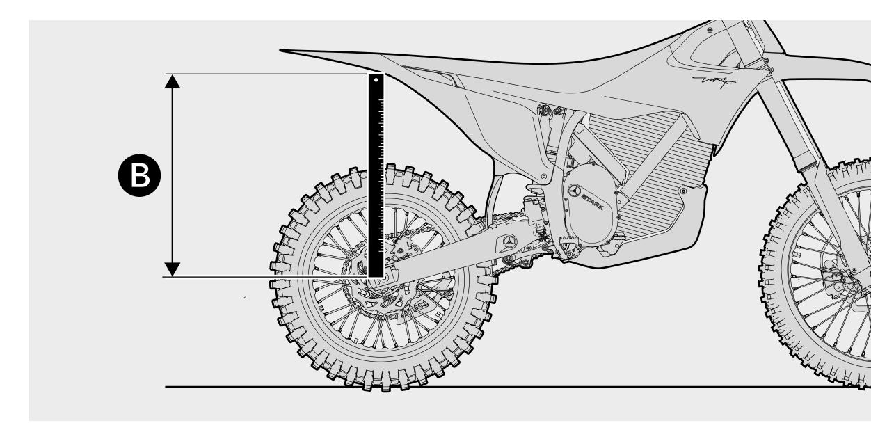
2 Place the bike with both wheels on the ground and measure the height B between the wheel axle and the SAG marking on the rear spoiler. Recommended value is: height A
