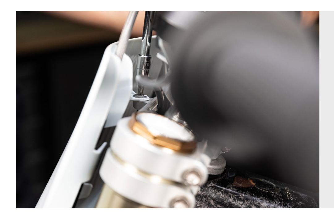
41 Loosen the foot peg spindle on the left side of the motorcycle and take it out.
