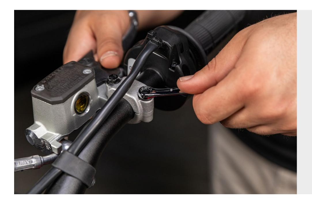
13 If your bike is equipped with rear hand brake instead of rear foot brake, repeat the previous step to attach the **rear hand**
