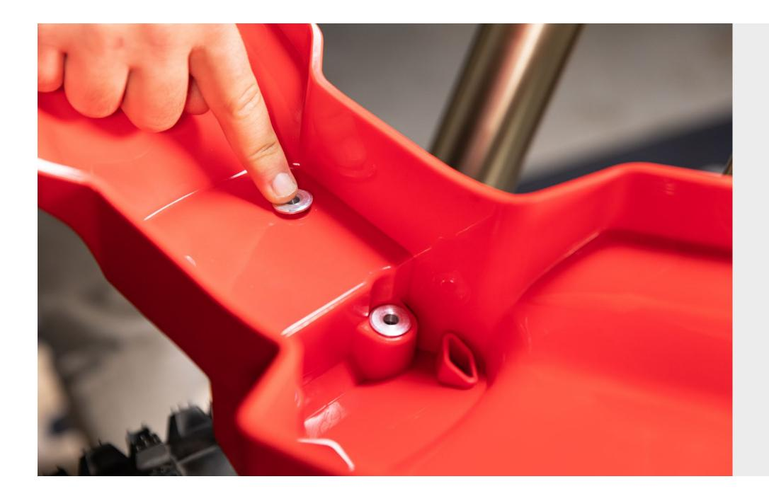
**37** Place the **front fender** in between the fork and align the notches in the **front fender** with the fastening points in the **frame**.
