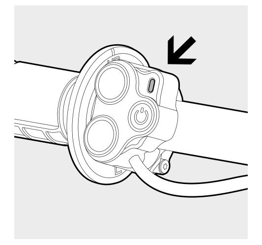
The control switch contains a **LED light** which can change color. Each color has a different meaning.
