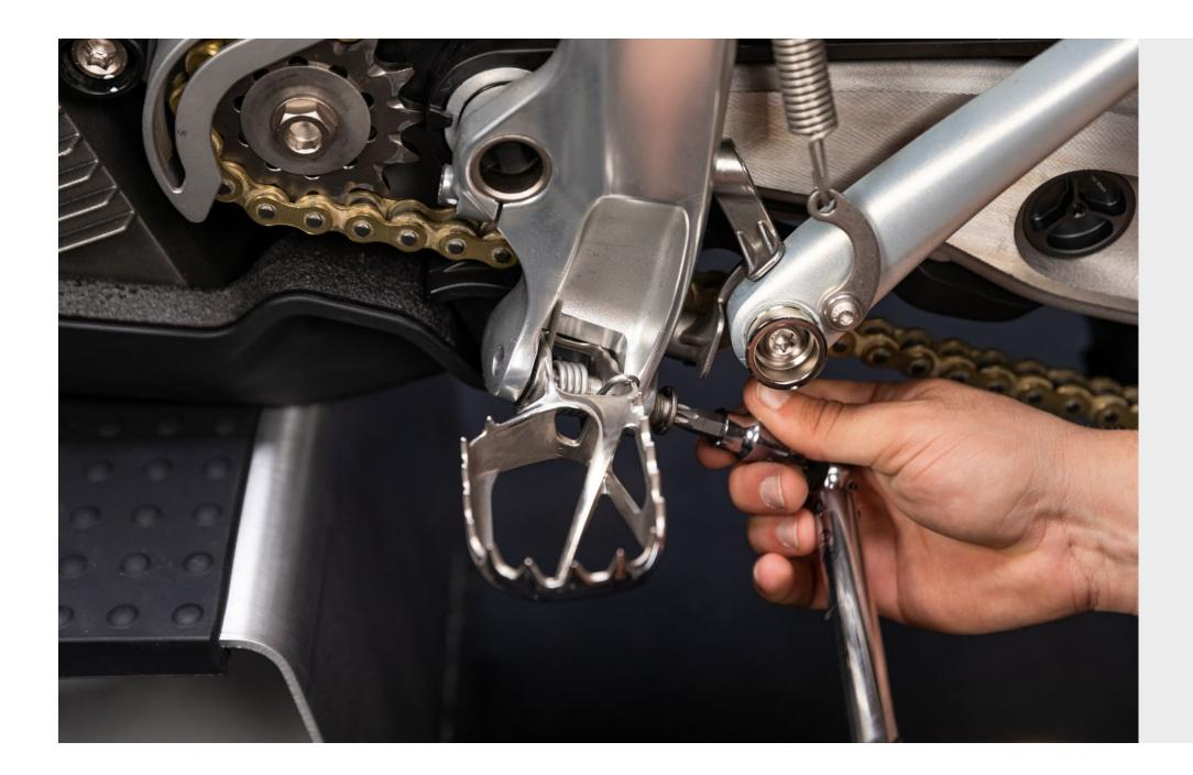
43 Push the foot peg spindle back to lock the left foot peg and tighten to 20 Nm.
