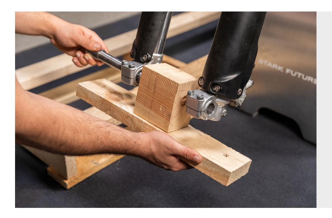
**28** While holding the wooden **front axle** holder, slide the front wheel axle out.
