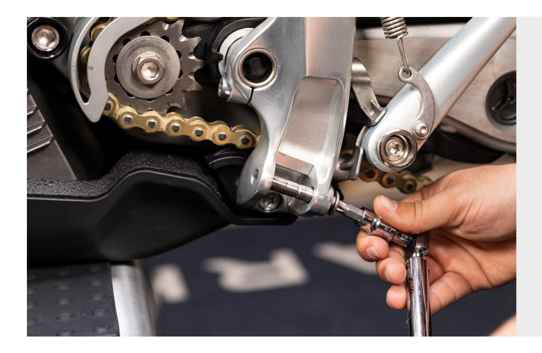
42 Place the left foot peg inside the recess on the left side of the motorcycle and gently push the foot peg inside the recess to align the shaft.
